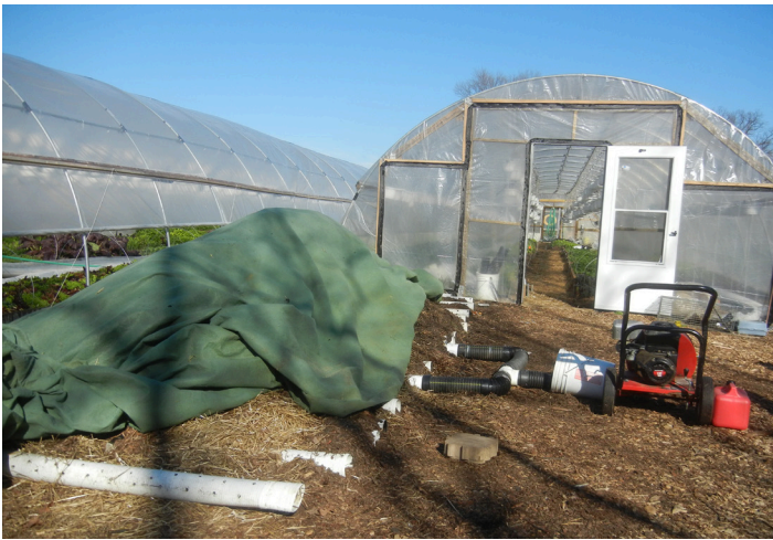
▲ The addition of a blower converts this otherwise passively aerated static pile into an aerated static pile at ECO City Farms in Edmonston, Maryland. Source: Institute for Local Self-Reliance.
